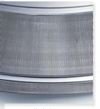
1 The classical inductive hardening process with its inductive head heats the needle bed gradually along its circumference. With this process, however, the needle bed is heated twice at the transition point: once at the begining of the cycle and a second time upon completing it. At this transition point, albeit miniscule, the needle bed has a lower hardness.
