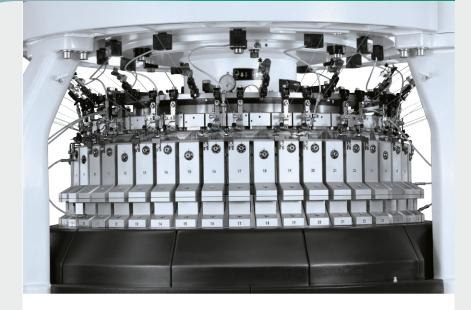
Proven and reliable electromagnetic single needle selection
